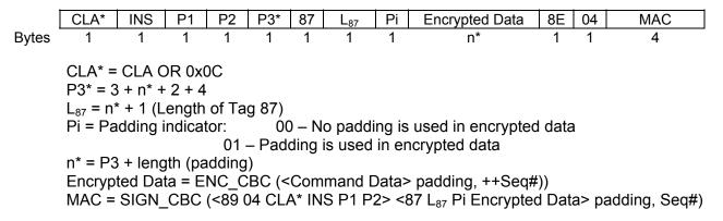
Since the maximum of P3\* must be less than 255, with the MAC, padding and the SMDO, the original P3 must be less than or equal to 240 bytes. Note that in the MAC calculation, the sequence number is not pre-incremented. This is because the encryption and the MAC will use the same sequence number with the encryption to be performed first.
