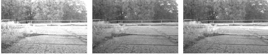
Fig. 6. Different exposure settings. The first image is captured with fixed exposure, the second with exposure control applied to the complete image and the last image was captures when camera exposure was controlled according to the top half part of the images.
