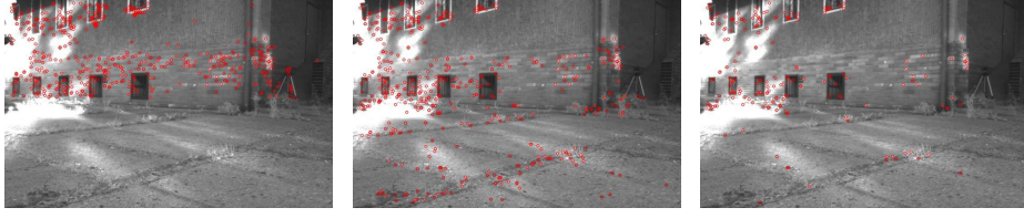
Fig. 8. Different setting of the keypoints detection: In the first image, 500 features are detected only from the top half. In the second image, the same amount is extracted from the whole image, and the last image has a fixed Hessian threshold, which results in feature deficiency.
