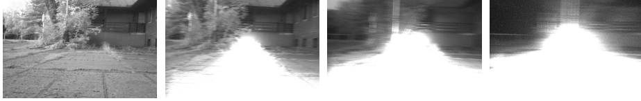
Fig. 14. Image blur caused by the lack of light at a sharp turn. The top left image is from the beginning of testing dataset, and the bottom right image was captured at the end of data collection.
